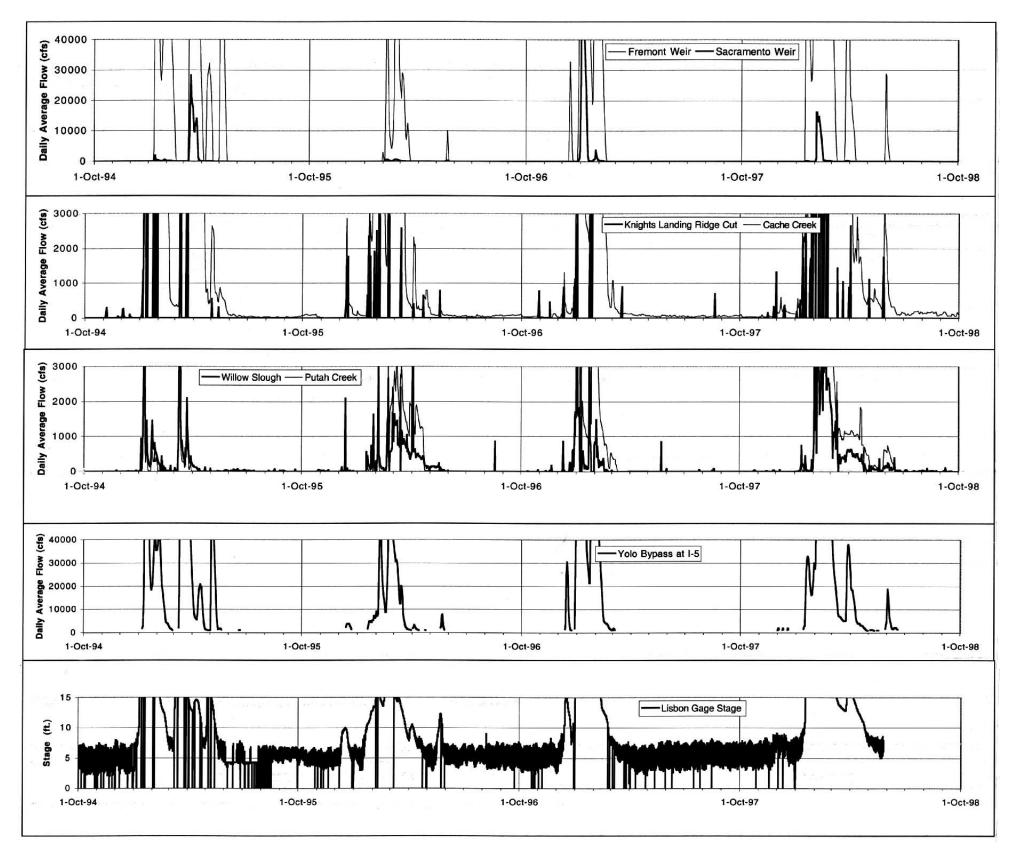
Figure 2-15 Hydrographs of Yolo Bypass Inflows and Stage at Lisbon Gage under Wet Conditions during Water Years 1995-1998 (Expanded Scale)
